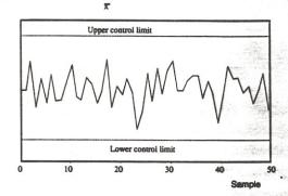
The centerline of this plot is typically the "grand mean" of the process defined as:
