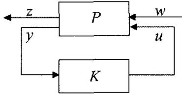
Figure 1. Generalized plant-controller configuration
