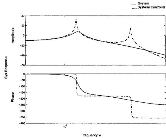
Figure 10. Results with positive real static controller
