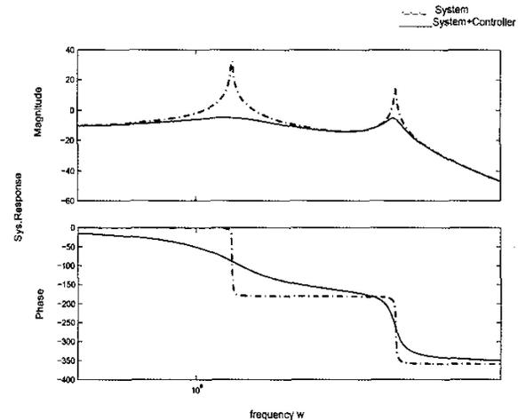
Figure 3. Results with positive real reduced order dynamic controller
