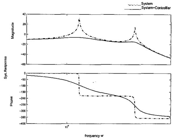
Figure 6. Results with positive real decentralized dynamic controller
