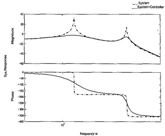
Figure 2. Results with positive real full order dynamic controller
