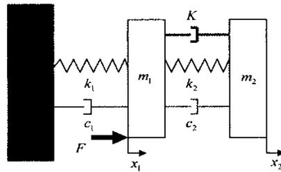
Figure 9. One controller between the masses
