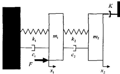
Figure 4. Controller on the 2nd mass
