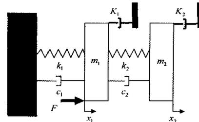
Figure 7. Two controllers on the masses
